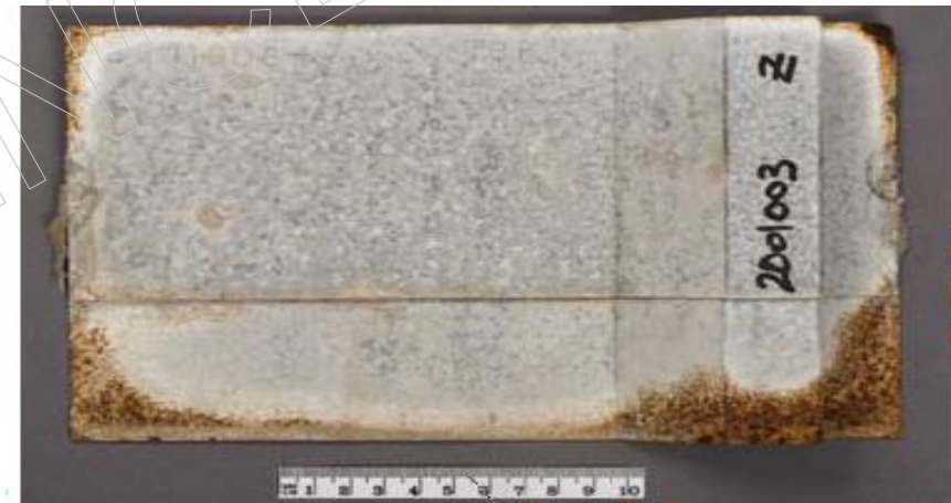
Galvanised Steel Z275 – 275g/m 2
