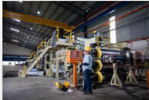
2. Core extrusion - 3 roller machine
