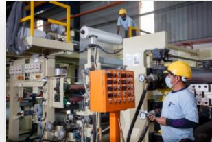
3. Adhesive film- go between core sheet & aluminum sheet
