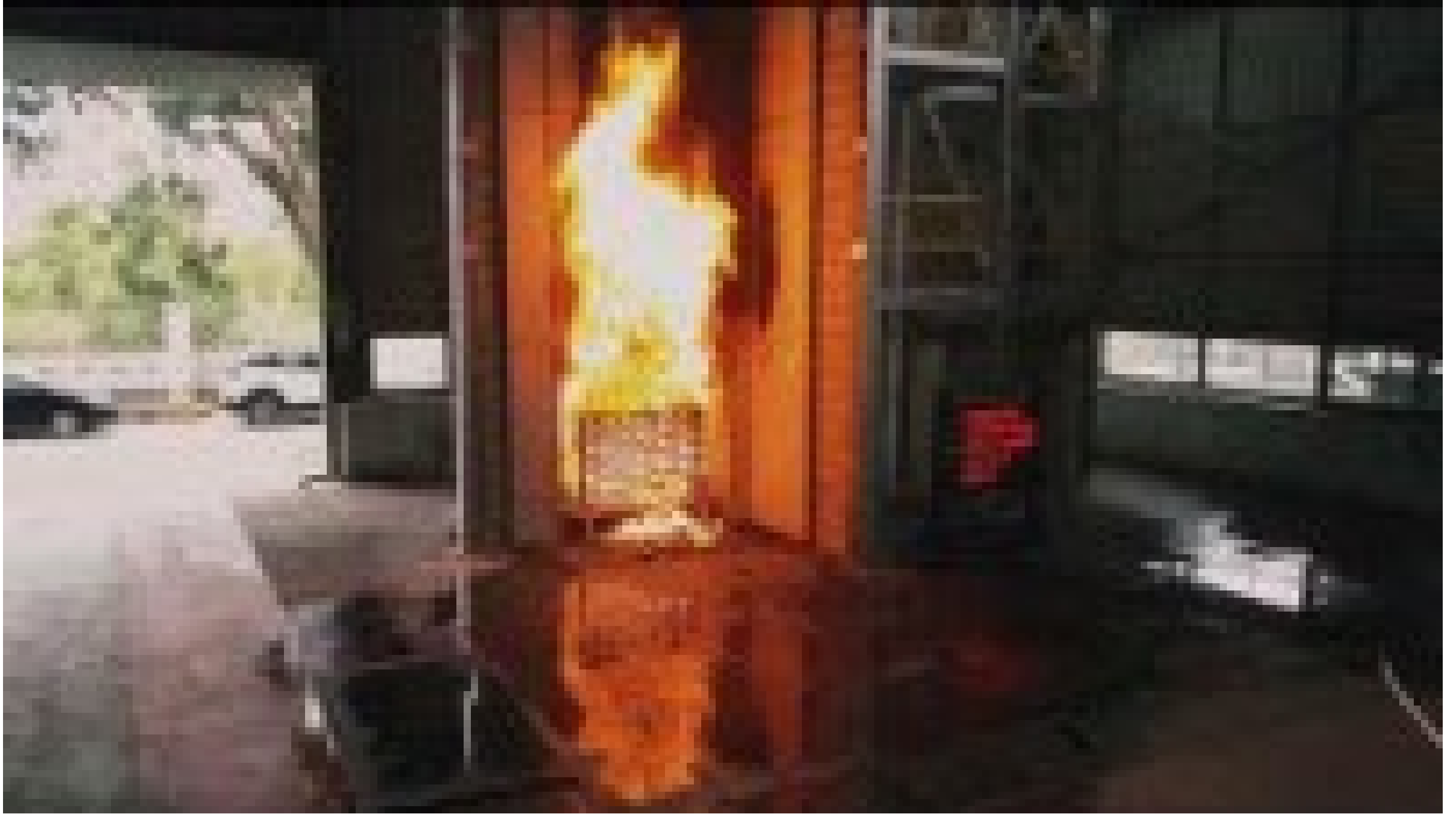
SIRIM Test Facility for BS8414
