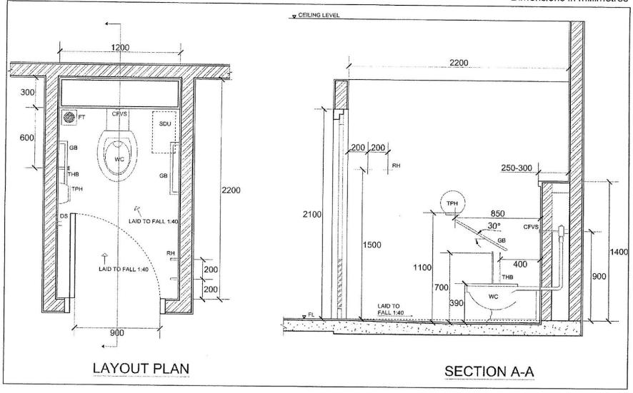
Figure F.3. Typical pedestal W.C. - Cubicle with grab bar
