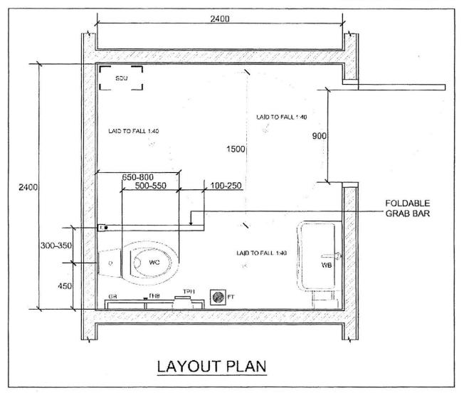
Figure F.12. Accessible toilet unit with toilet pan at side
